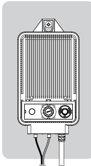
Attach the transformer to the wall by using the hook. See requirements (p.1)
